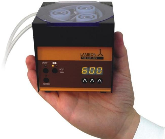
LAMBDA PRECIFLOW, MULTIFLOW, HIFLOW, MAXIFLOW and MEGAFLOW laboratory peristaltic pumps are specially designed for long term continuous processes with flow rates from 0.2  $\mu\text{l}/\text{min}$  to 60'000 ml/hour. High precision, reproducible and long term stable flow rates are achieved with the quartz driven motor and unique tubing compression technique in the large pump head.
